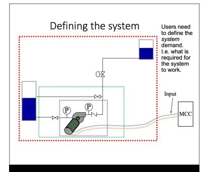
Fig. 2 Efficiency of a pump measured on a component basis (purple box) based on the ratio between the pump's input and output. The system view includes a re-circulation line as shown by the green box. Looking at the complete pumping system using a total system approach is illustrated by the red box.
